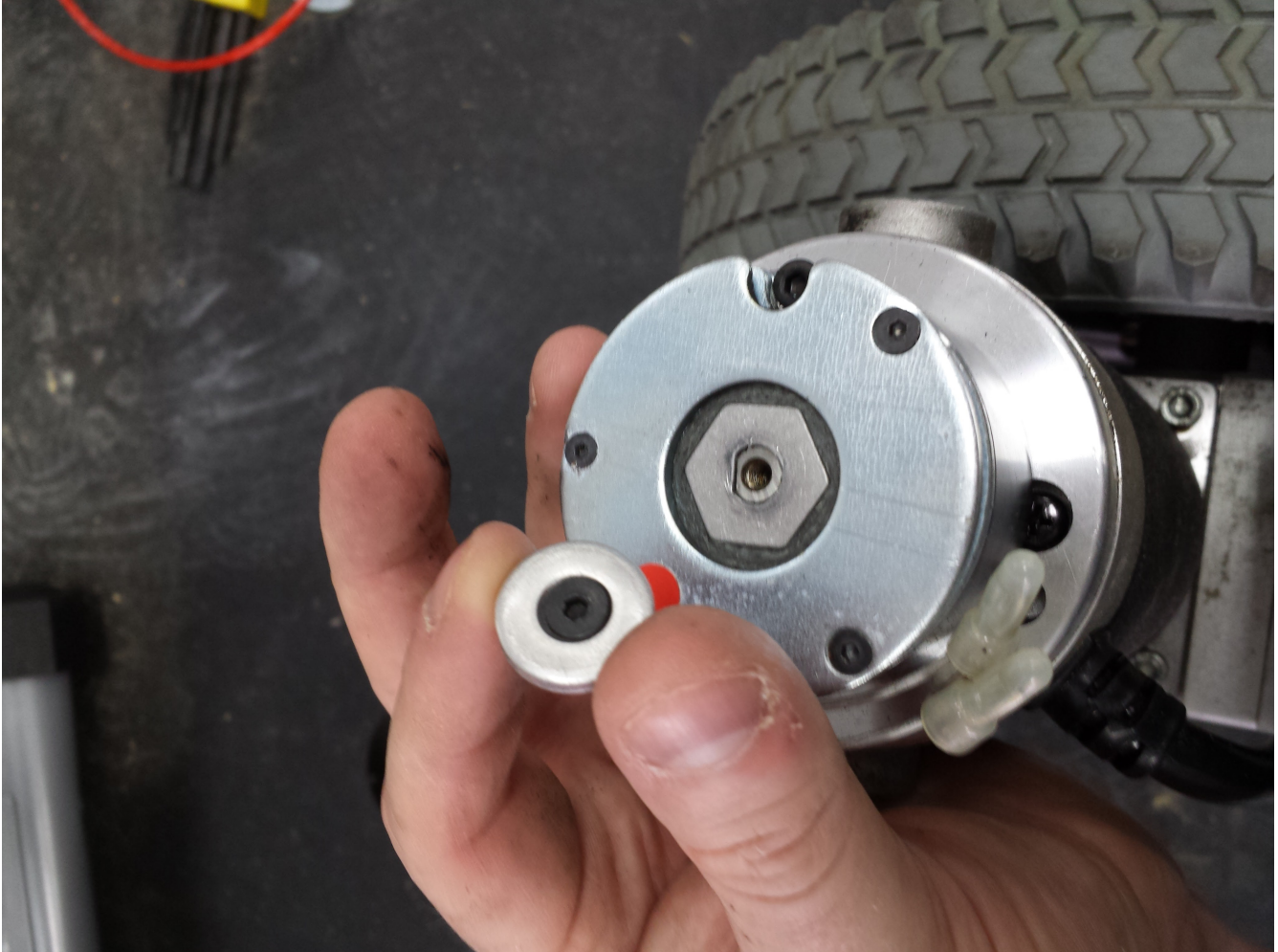
Illustration 4: Remove the center retaining washer by unscrewing the center bolt
