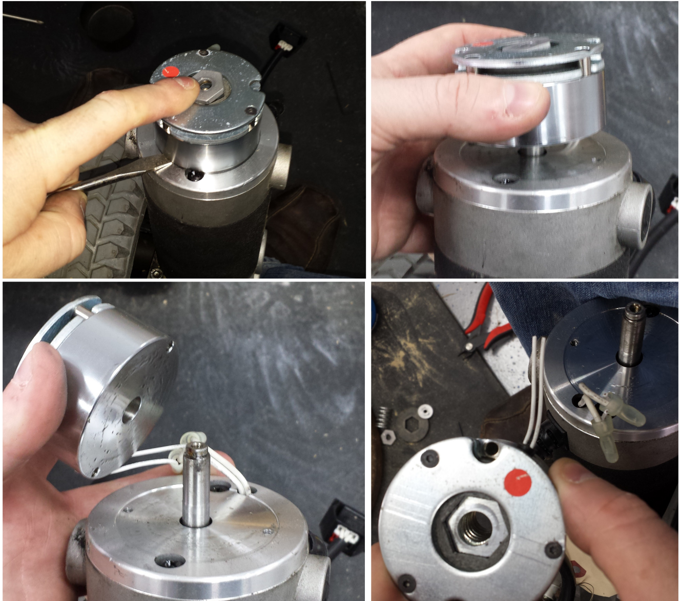
Illustration 6: Pry and lift off the EM brake
